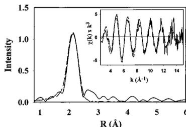
**Figure 1.** Experimental vs simulated Fourier transform and EXAFS (inset) for N-MNKp with multiple site occupancy ( $n \geq 4$ ). The Fourier transform of the  $k^3$ -weighted EXAFS data was corrected for the Cu–S phase shift. Solid lines represent experimental data; dashed lines represent the best fit with two S at 2.16 Å ( $\sigma^2 = 0.0044$  Å<sup>2</sup>), EXCURV98 simulation.
