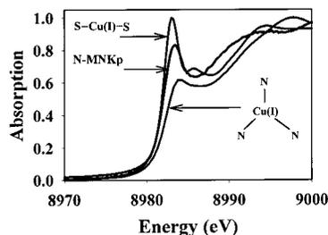
**Figure 2.** Cu K-edges for N-MNKp and model complexes: 2-coordinate model compound  $[\text{N}(\text{C}_3\text{H}_7)_4][\text{Cu}(\text{SC}_{10}\text{H}_{13})_2]$  (thick);<sup>21,30</sup> Cu(I)–N-MNKp (medium); 3-coordinate model compound  $[(\text{Me}_2\text{Im})_3\text{Cu}(\text{I})]^+$  (thin).<sup>28</sup>
